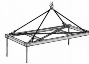
Example of container lifting using a lifting beam fitted with hooks, shackles or manually coupled locks.
